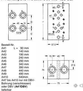
DBV=RPEC-FAN (Typ 9911-04A-G01) Fa. Sun Hydraulik
